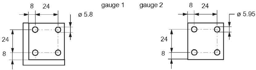
Fig. 18.86 Functional gauge according to the example in Fig. 18.85
